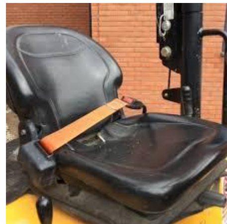
Dumper lap belt in incorrect position
