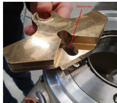
Change-over selector actuator, "batman" piece
