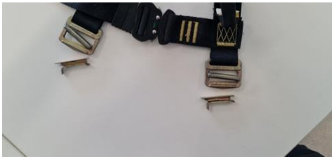
Figure 2 - Failure of the latches on the straps of the harness.
