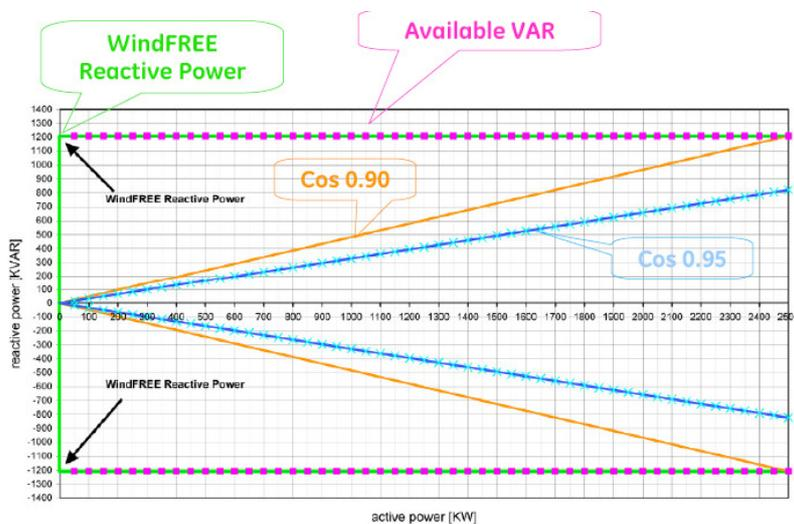
Figure 10 – Reactive Power Capability for One WTG Type – Includes Synchronous Compensate Mode
