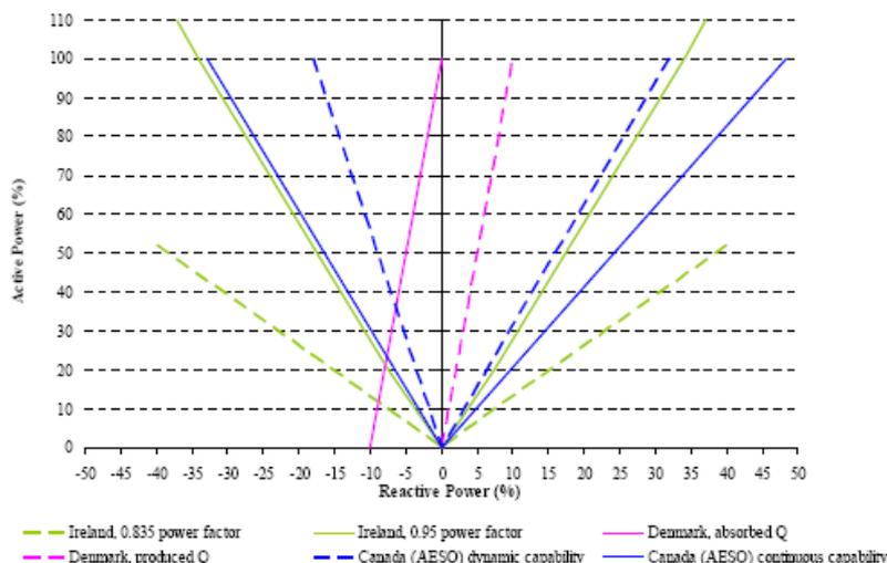
Figure 8 - Comparison of Reactive Power Requirements from Various Grid Codes
