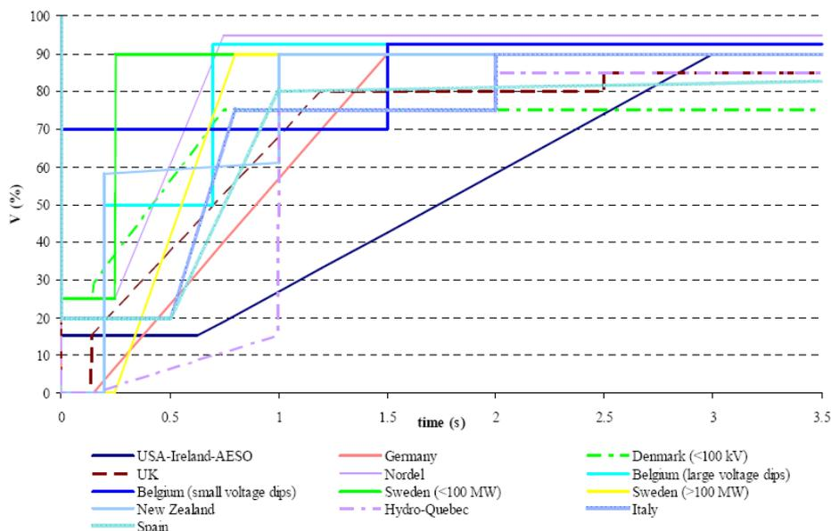
Figure 7 – Various International Codes for Low Voltage Ride Through
