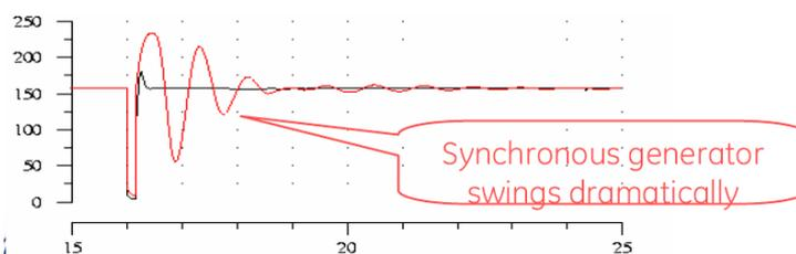
Figure 9 – Comparison of Conventional Generator with Full Converter Output WTG
