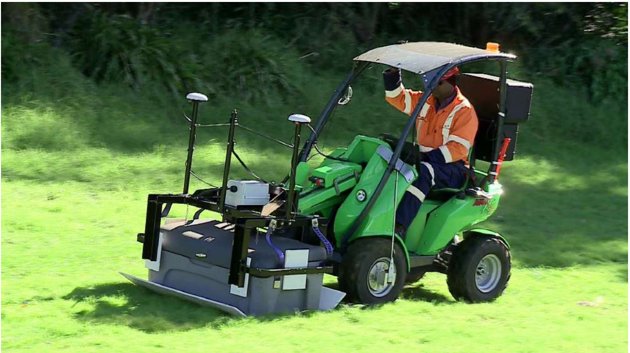
Figure 5 – PAL-GPR capture vehicle in operation
