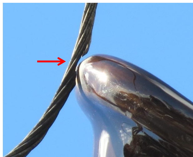
Fig. 2 Flash-over and heavy erosion caused by a jumper touching insulator
