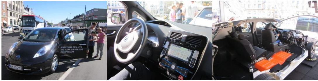
Figure. 2: The Nissan Leaf BEV including a view of the battery pack (orange)
