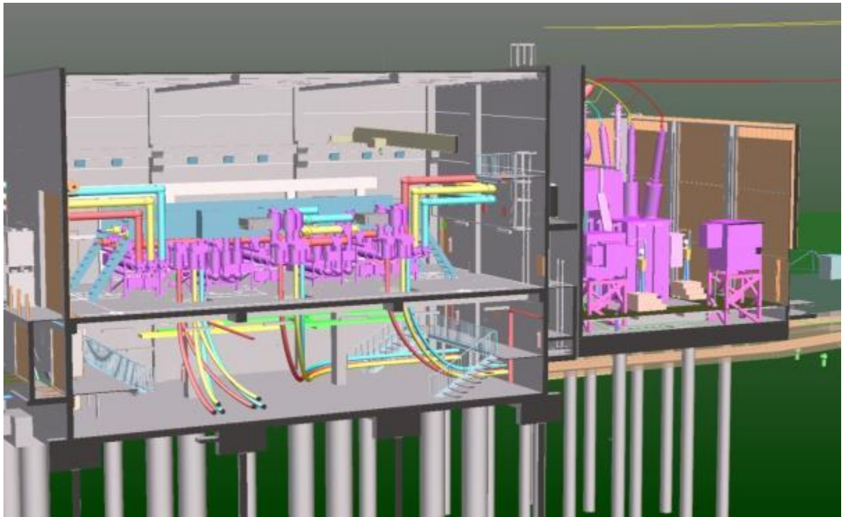
Figure 6 – 3D Model of GIS floor, HV Cable Basement and Transformer enclosure
