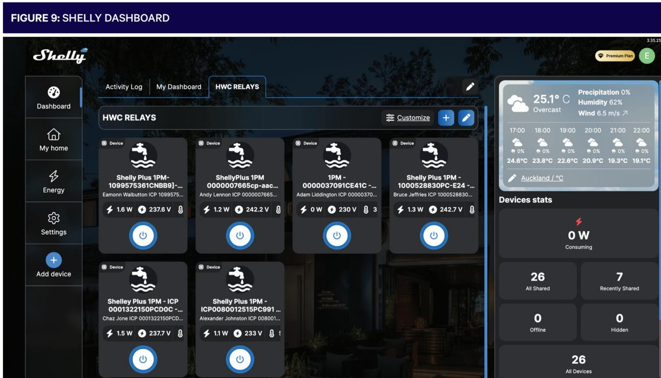
Hot Water Control (HWC) Relay Dashboard showing Shelly products connected via the Shelly application interface for products located in electricians (customer) homes.
