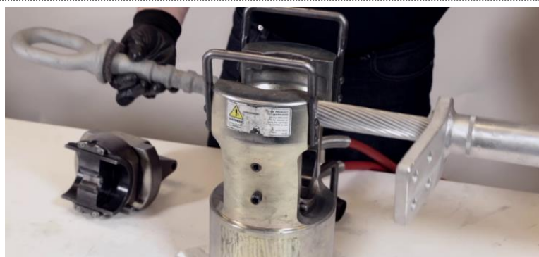
Figure 1 - press-head dead-ending conductor joints.
