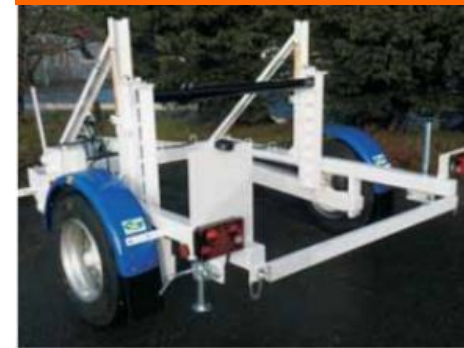
Example of a cable drum trailer
