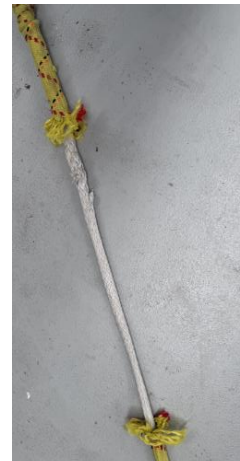
Missing sheath on lifting line
