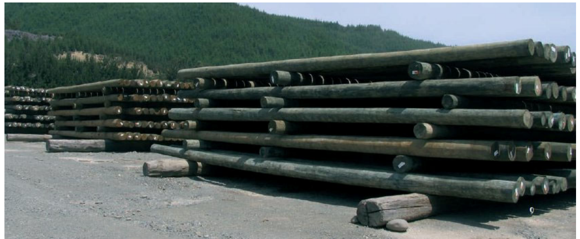
Twelve months in the yard is what turns a chemically-treated pole into a dimensionally stable one.
