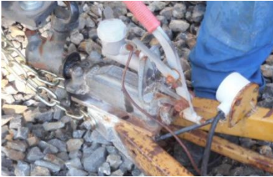
Re-enactment of how the injured employee's foot was trapped
