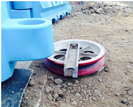
The failed pulley block
