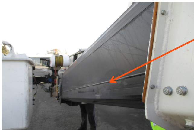
Photo 1: Steel boom section with failed weld
