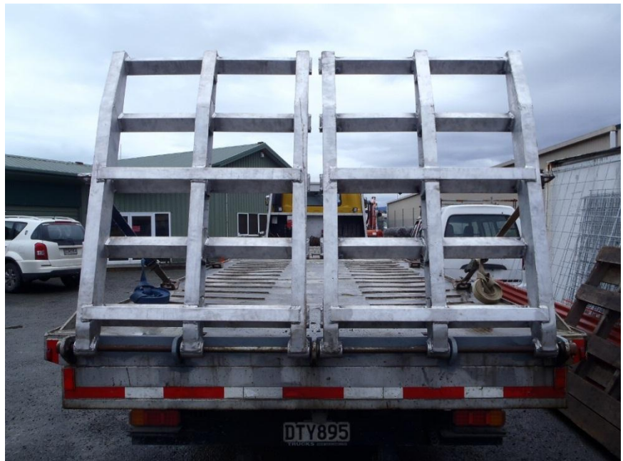
Modified Transporter Deck and Ramps
