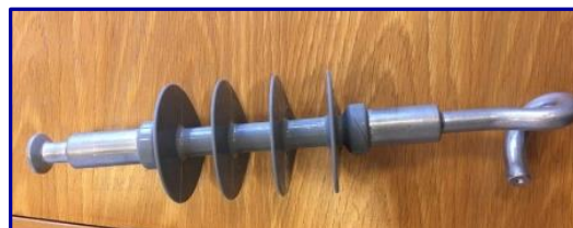
Figure 1. Faulty pigtail OHL Insulator
