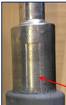
Figure 4. Correctly Compressed Mosdorfer Insulator
