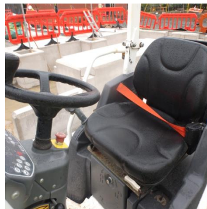
Bypassed Restraining System
