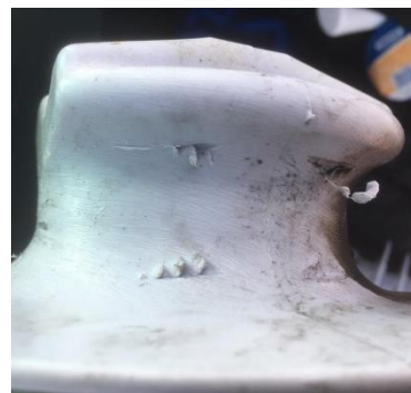
Fig.3 – Marks on failed insulator
