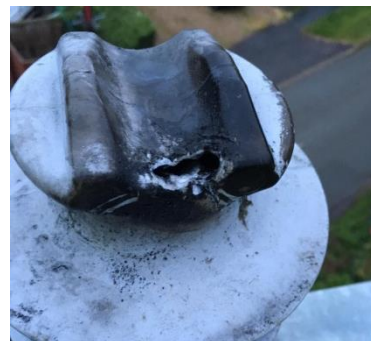
Fig.1 – 1 st failed pin insulator
