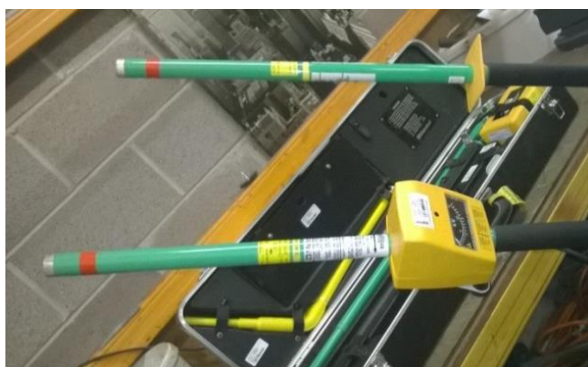
Moving coil type HV Voltage Indicator and Phasing Rod
