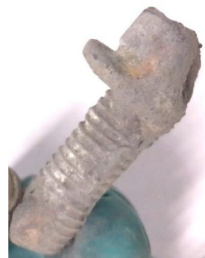
Fig 1: Bolt found inside LV board
