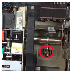
Fig 3: Area of defective drive pin from Schneider defect notification
