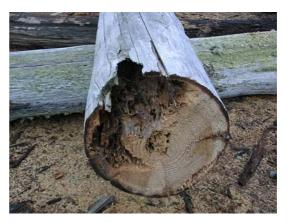
A recently discovered rotten larch pole (above) in which the area of rot concerned was at two metres above the ground level. This demonstrates the importance of all pole security checks before any climbing is attempted.
