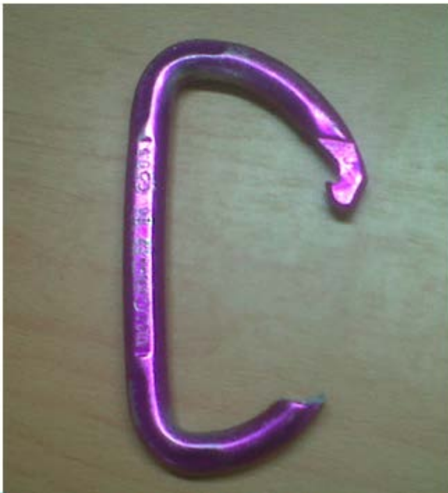
PICTURE OF FAILED KARABINER
