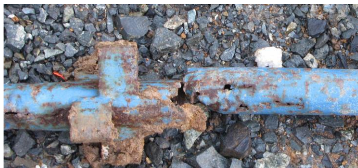
Photo of the broken scaffold tube
