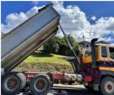
A transportation subcontractor engaged to transport hard fill between two sites in Newlands left the truck’s Power Take-Off (PTO) engaged post load release. PTOs allow trucks to power equipment like hydraulic lifts, pumps, or other tools, without needing a separate power source.
