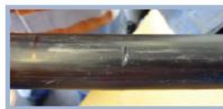
Without KPI – Damage to Sheath
