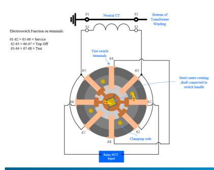
There are several ways that a high voltage can appear across an Electroswitch CT wafer. One is primary current flowing in the CT with the switch in "Test" position and the TP installed shorting link missing.
