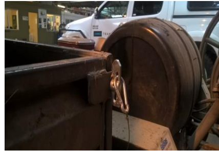
Picture 2: Latch with retaining clip and tether installed
