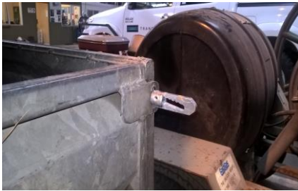
Picture 1: Standard trailer latch in open position
