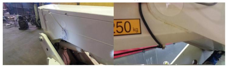
**Event Details:** During periodic boom inspection and certification, the inspector identified a failure in a weld in the lower portion of the boom, with a crack like indication detected at the weld toe extending for approximately 220mm. Further inquiries are being carried out to determine the cause of the failure. The EWP, which is two years old, has been removed from service until repairs and/or replacement of the failed section has been initiated.
