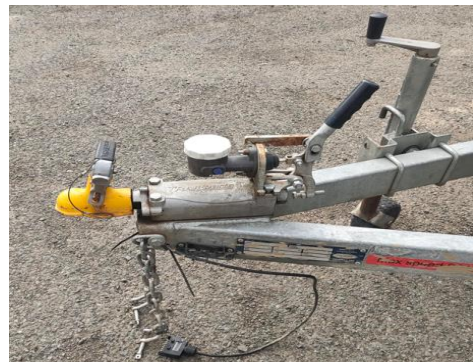
Figure 2 Trailer brake locked out.
