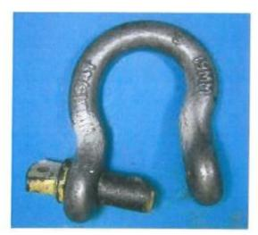
**Event Details:** Crane Association NZ have issued a product safety recall on all "IWR BOW Shackles and Pins with the markings as shown above, the range of recall are rated at working limit WLL 1.0T to WLL 25T. There is a concern that the harness of the Shackle Pin maybe prone to fatigue crack initiation from stress raisers. This could result in fatal injury and or damage to the user or surrounding area.
