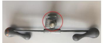
Figure 1: shows incorrect alluminium alloy clamp L044606 removed from conductors, corrosion resulting from dissimilar metals can be seen on the clamp.
