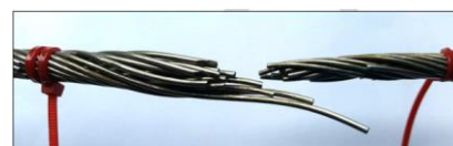
Photo 1: The two broken cable ends with loose strands rewrapped (lower end on left, top end on right).
