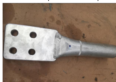
Figure 3. Example of lug with correct 3mm hole
