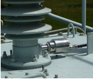
Figure 11. Tap sensor for C, tgδ, transients and PD measurements
