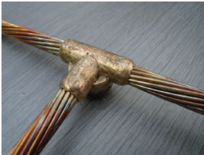
Copperbonded steel conductor at 30% conductivity Suggested Connection methodology: Exothermic- CADWELD
