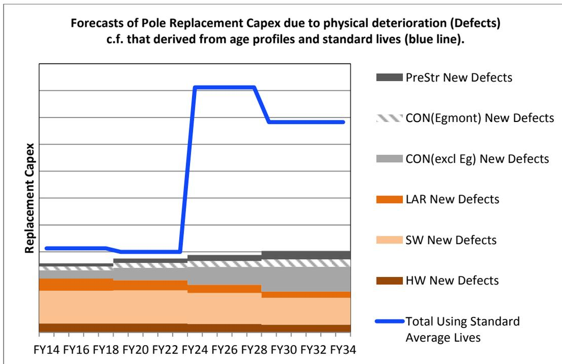
*Figure 11: Projections of new defects expected based on derived Survivor Curves together with comparison to that derived from age profiles and standard lives*
