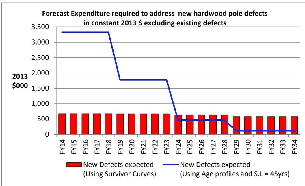
Figure 8: Example replacement capital cost forecasts using survivor curves (red) c.f. age profiles and a standard life (blue)
