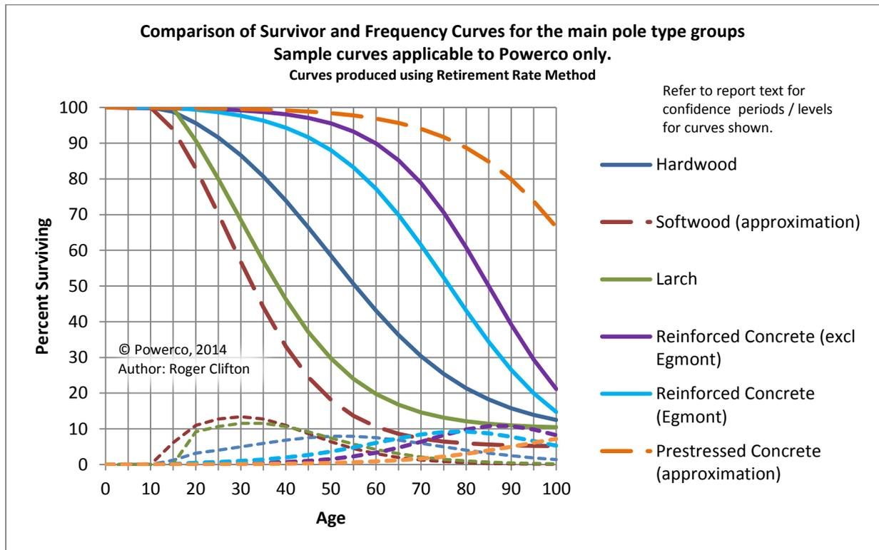
Figure 10: Comparison of Survivor Curves for Powerco’s main pole types derived using the Retirement Rate Method
