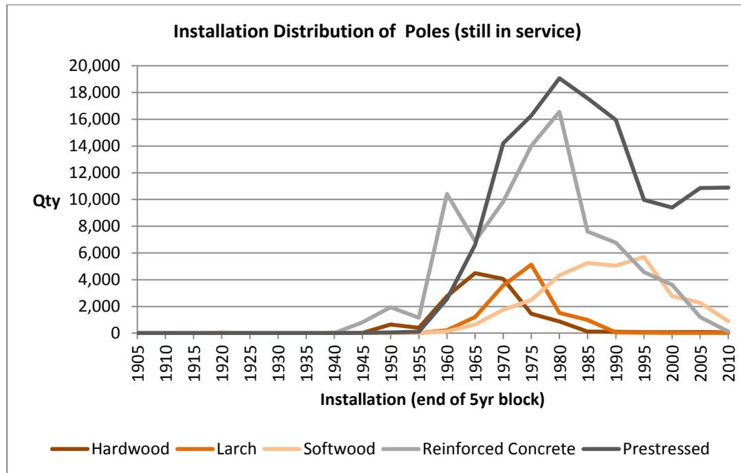
Figure 9: Pole Installation Distribution
