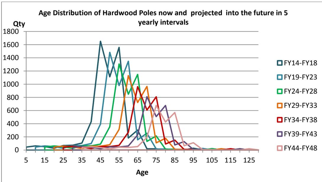
Figure 7: Forecast movements in hardwood pole age distributions using derived Survivor Curve
