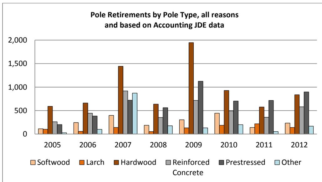
Figure 2 Pole retirements by pole type
