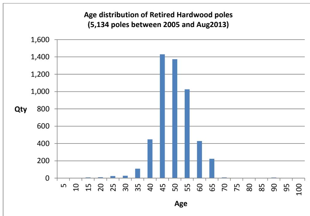
Figure 6 Age distribution of Powerco's retired (disposed) hardwood poles
