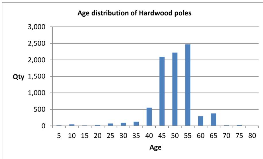
*Figure 3 Age distribution for Powerco's hardwood poles inspected up to Aug 2013*
