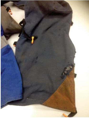
Condition of chaps after incident
